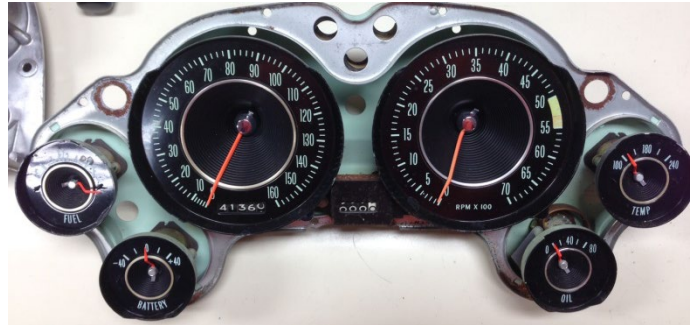
OEM Gauges Removed
